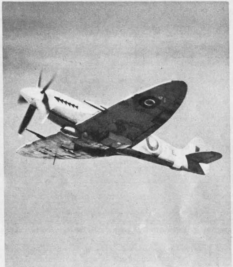
Three air scoops break the under surface of the wing. One is set at leading edge of wing beneath the fuselage; two others are outboard.
